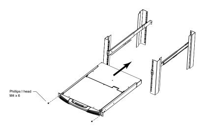
5. Slide the rear attachment sliding brackets along the slide bars until they contact the rear of the switch, then use the screws supplied with this package to attach the bars to the rear of the switch (tighten the screws all the way).
